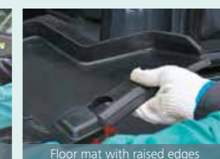
Floor mat with raised edges Floor mat's raised edges help keep the cab floor free of mud, simplify cleaning.
