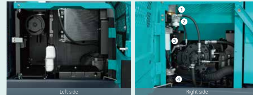
Left side Simple layout for easy access to radiator and cooling system elements
