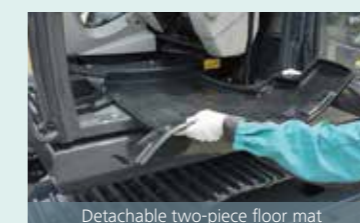
Detachable two-piece floor mat Detachable two-piece floor mat with handles for easy removal. A floor drain is located under floor mat.
