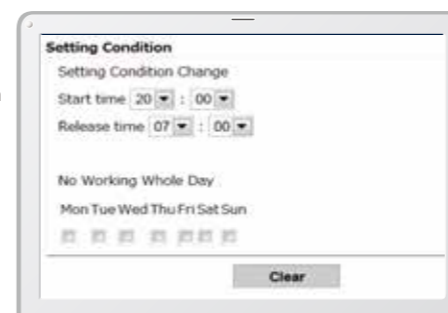
Engine start alarm outside prescribed work time
