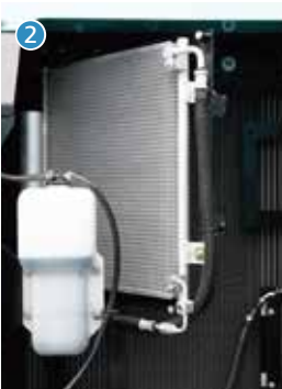
Openable airconditioner condenser
