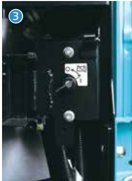
Battery shut-off switch
