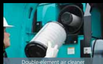
Double-element air cleaner
