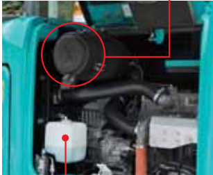
Radiator reservoir tank
