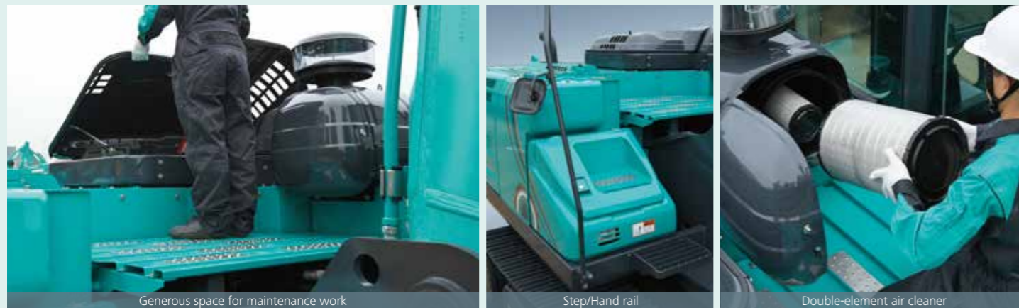
Generous space for maintenance work
