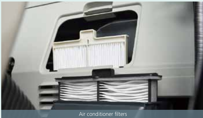
Air conditioner filters
